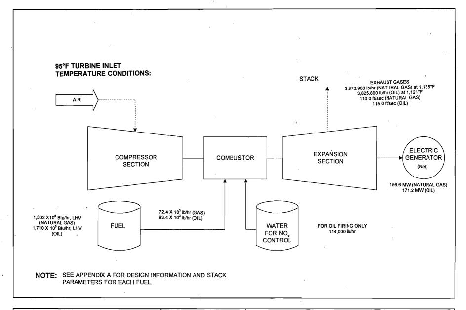
Figure 2-2 Simplified Flow Diagram of Proposed "F" Class Combustion Turbine Baseload, Summer Design Conditions
