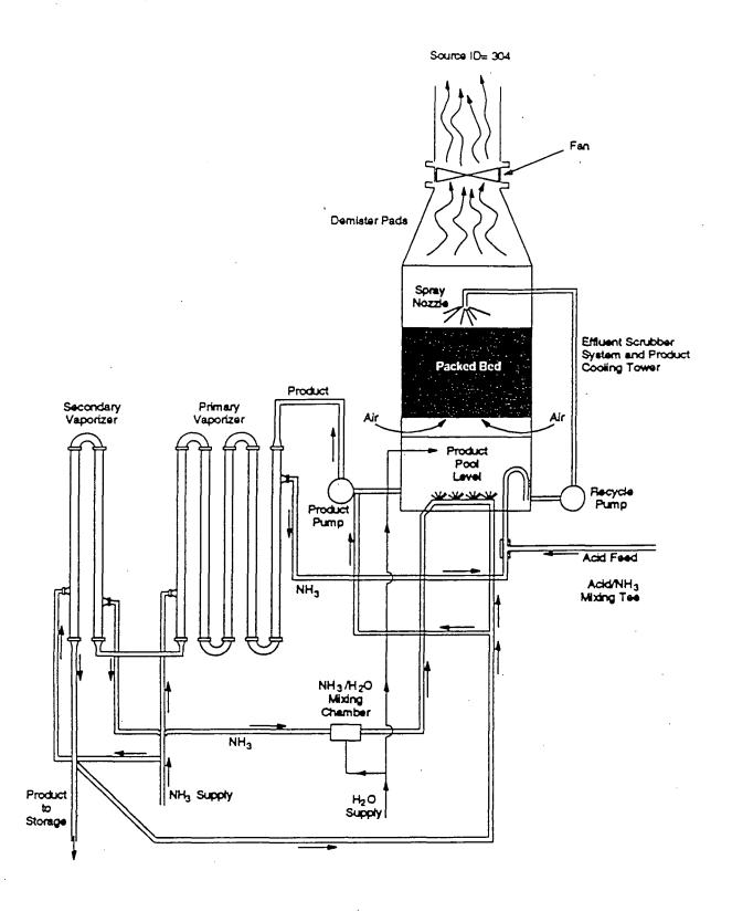
Figure 2.5-5. Schematic Diagram of Ammoniated Polyphosphate Production Process
