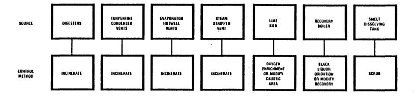
FIGURE 3-1. NONCONDENSIBLE GAS (NCG) EMISSION SOURCES AND CONTROLS
