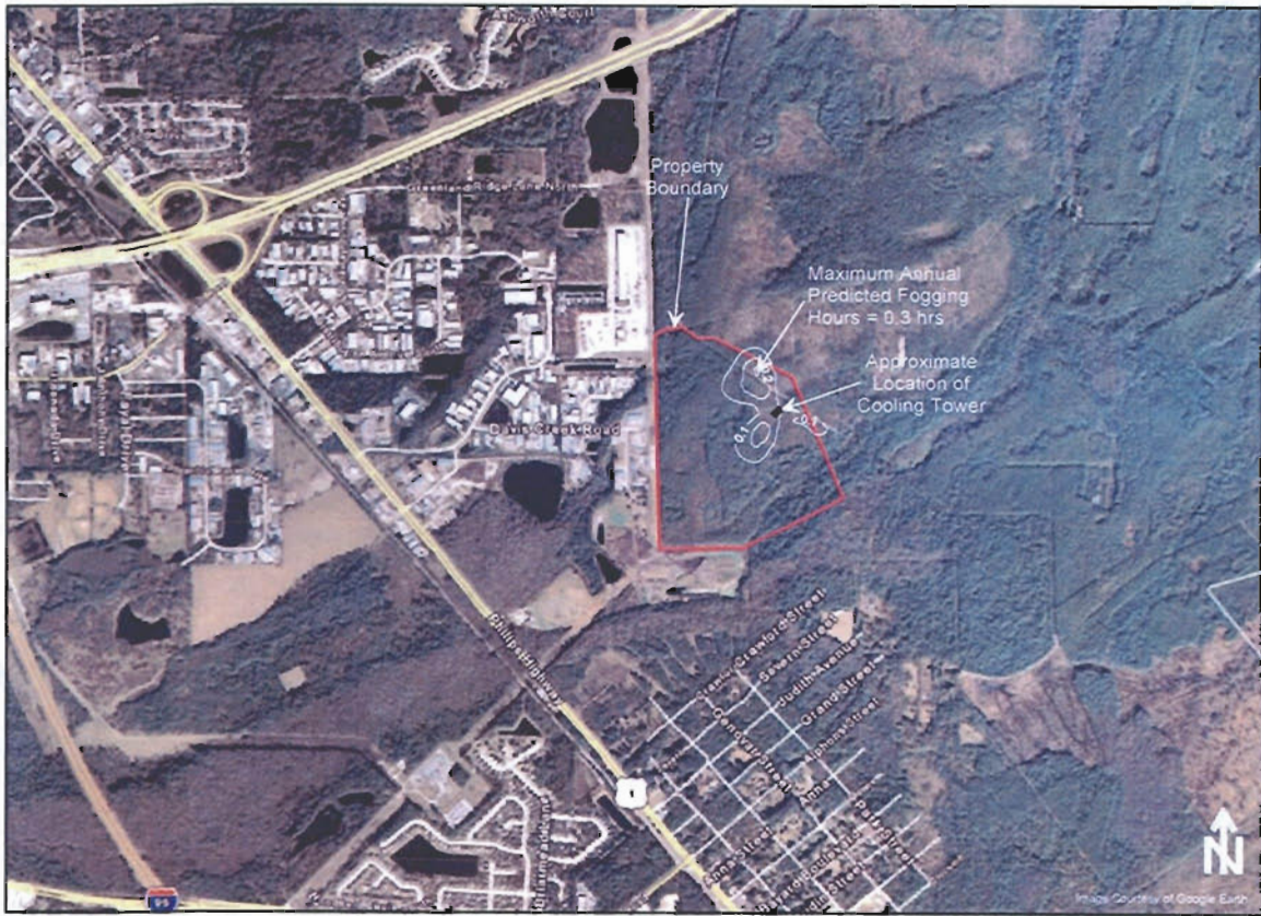
Figure 5.1-1 Predicted Cooling Tower Induced Fogging
