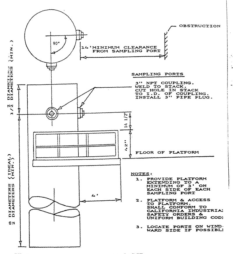
IF THE STACK DIAMETER IS TOO LARGE TO TRAVERSE FROM ONE PORT, 4 SAMPLING PORTS AT 90° APART MAY BE USED TO TRAVERSE THE STACK. THIS AVOIDS USING A LONGER PROBE WHICH MAY CAUSE SAGGING
