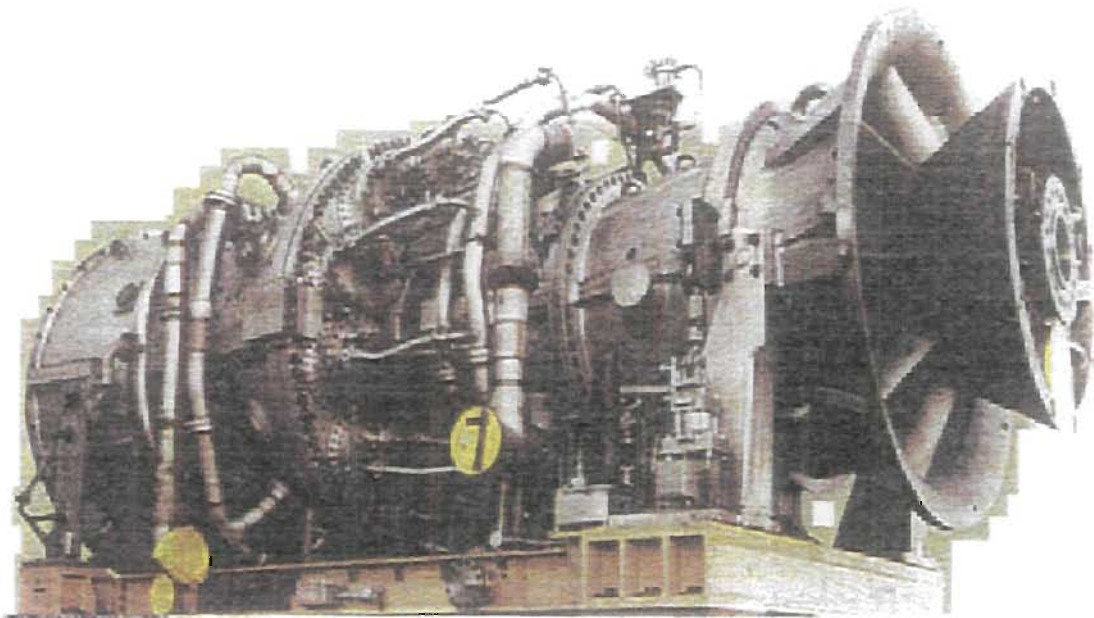
Figure 2 - Photograph of General Electric MS 7001FA Combustion Turbine
