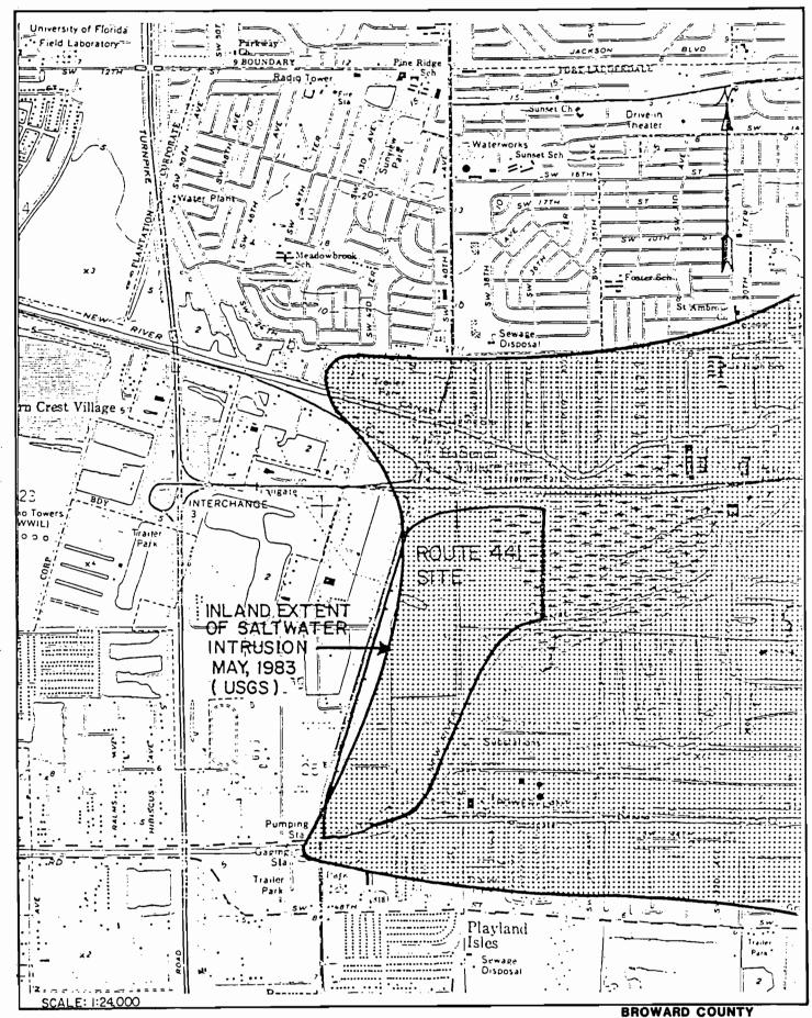
RESOURCE RECOVERY ROUTE 441 SITE 1,000mg/I ISOCHLOR FOR BISCAYNE AQUIFER Well S830, which is located on the Florida Power and Light Company property (southeast of the site), is screened at about 130 feet and showed chloride concentrations in the range of 1,000 to 3,500 mg/L.
