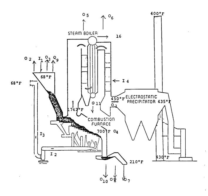
Efficiency = Net Heat in Steam X 100 Net Avail. Heat Input
