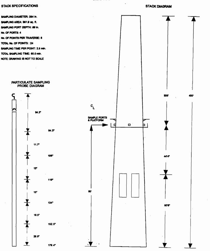
Access to the sampling ports is provided by a ladder. Channel iron with a trolley system is above each port for probe support. AC power is available on the platform and at the base of thestack.
