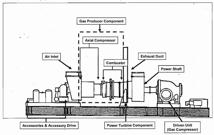
Engine 1607 is one of the new model gas turbines, a Cooper-Rolls Model 501-KC7-DLE. These units have experienced some initial startup problems including blower bearing failures, high vibrations, and compressor bleed valve malfunctions. The gas generator has previously been replaced under the initial air construction permit. However, construction of Engine 1607 is complete and the authority to construct has expired. The unit is now included under current Title V air operation
