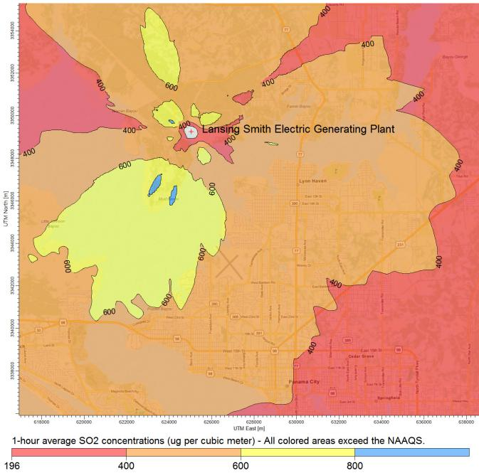
Figure 2 - Local View of Lansing Smith Impacts Based on Allowable Emissions
