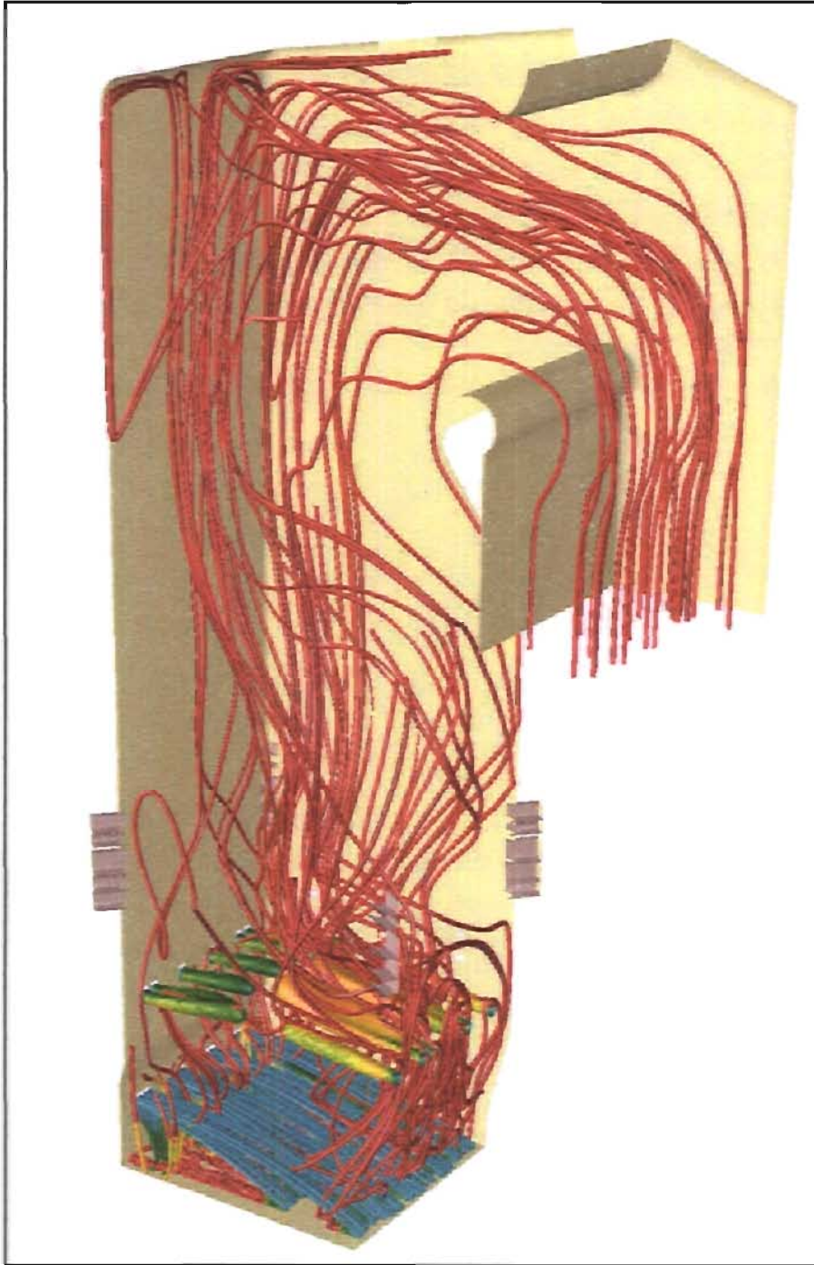
Fig. 9 Bark Particle burning trajectories colored by state
