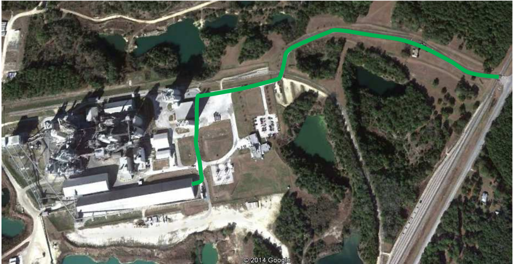
FIGURE 1. AFM VEHICLE TRANSPORT ROUTE (0.65 MILES EACH WAY).
