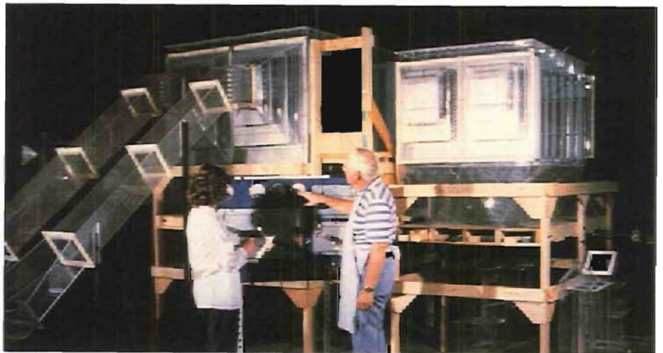
Gas flow model test – Baltimore Technical Center.
