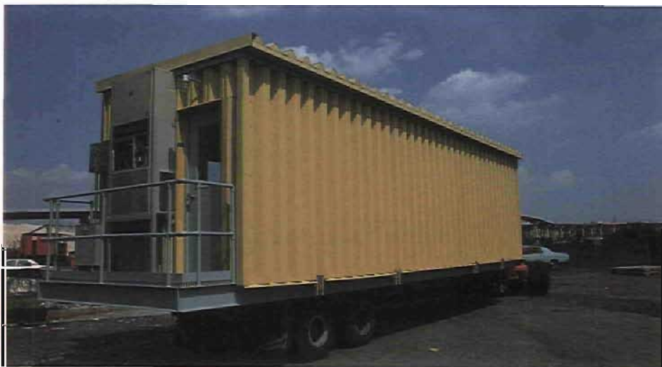
Prewired and preassembled climate controlled precipitator control house.
