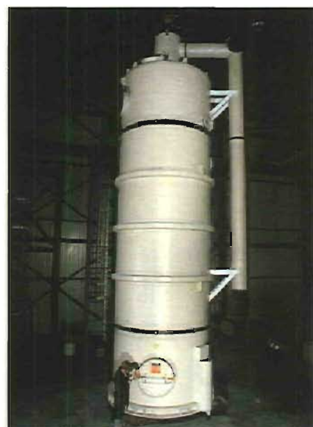
One 36 tube FRP tubular fibre glass acid mist precipitator — Barrancabermeja, Colombia.
