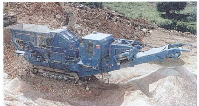
▲ A 428 Trakpactor working on a construction project producing crushed limestone at 400 tonnes per hour.
