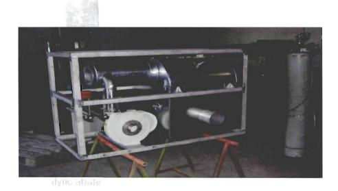
The needed extract for maintaining the airflow through the Catalytic Abator Plant for conversion of ETO is supplied from a fan on the inlet duct to the abator.
