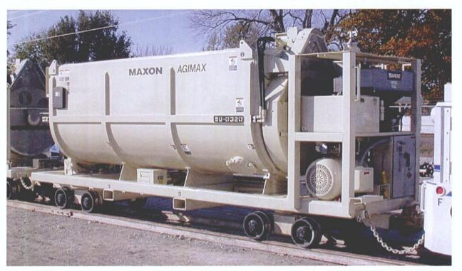
The new **Maxon Agimax** is designed to transport, agitate and place concrete for low profile underground applications, where discharge heights will not allow a full hoisting body similar to the **Maxon Agitor**. When working in small-bore tunnels, the Agimax offers many advantages not available with conventional agitator cars.
