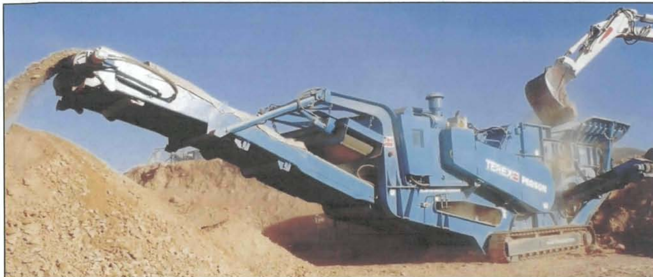
Above photograph features a 1412 Trakpactor fitted the with optional side conveyor and magnet.
