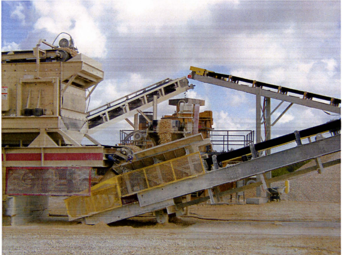
Crusher Input Conveyor and Crusher (Background) Screen and Crusher discharge Conveyors (Foreground)
