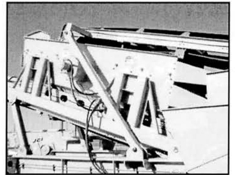
Vibrating screen features hydraulically driven adjustable speed and stroke.
