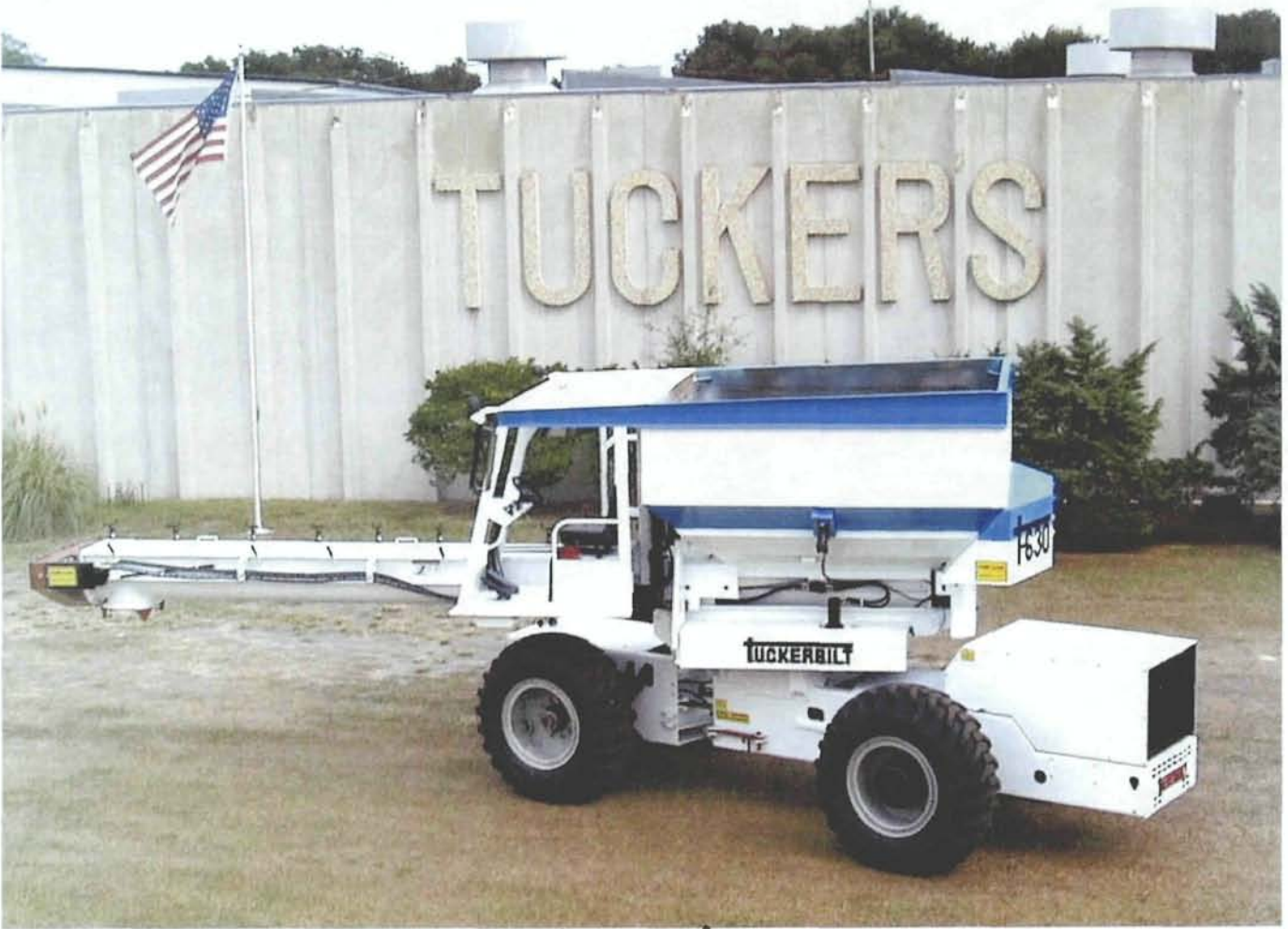
Concrete delivery vehicle
