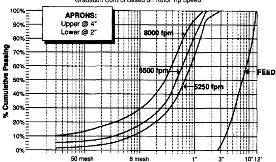
\* Capacity depends on feed size and gradation, type of material, etc.
