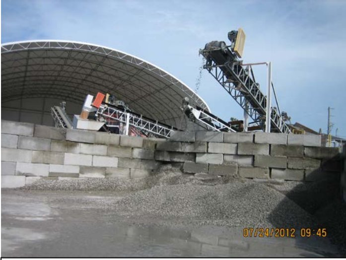
Photo ID No: IMG_466 – In this photo, Hopper No. 2, Screen No. 2 (Red), Belt No. 5(into hopper), and Pile Conveyor No. 3
