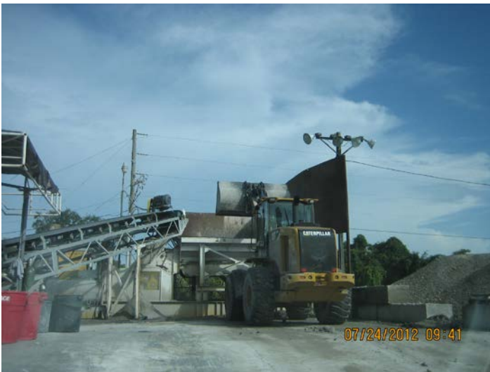
Photo ID No: IMG_458 – B. E. T. ER Mix, Inc. Non-Metallic Mineral Processing Plant crusher hopper loading in progress.
