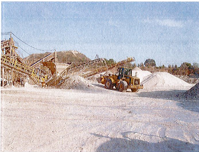
Photo ID No. / Date / Time: Picture 07 03-15-2011 Hopper and Conveyor Belt to Canica-Jaques Crusher
