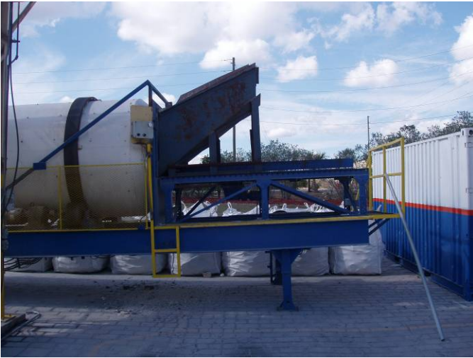
Photo ID No: 1050372_Photo_01_24_2012-24 Time: Approx. 12:20 PM Back view of paver tumbler, where pavers are loaded into tumbler. Camera facing approx. W.
