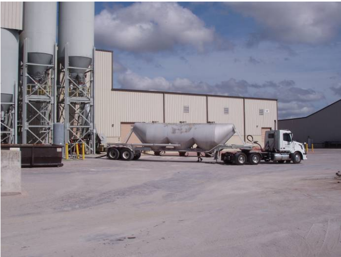
Photo ID No: 1050372_Photo_01_24_2012-10 Time: Approx. 11:45 AM White cement truck outside of Plant 4. About half of the white cement in this truck was used to fill the Plant 1 white cement silo (EU002) during the second VE test at the facility on 01/24/2012, and the remaining contents of white cement in the truck were used to fill the Plant 4 white cement silo (EU012) during the third VE test at the facility on 01/24/2012. Camera facing approx. NW.
