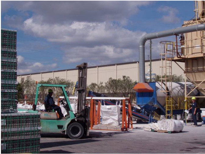
Photo ID No: 1050372_Photo_01_24_2012-16 Time: Approx. 12:20 PM An operator waits to transport a filled paver bag and another operator controls the paver tumbler machine. While the fork-lift is used to deliver a filled bag to a storage area, the conveyor belt shifts to fill the second bag with pavers and an operator places an empty bag on the rack to be filled.
