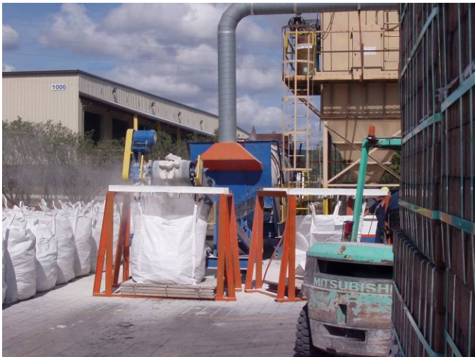
Photo ID No: 1050372_Photo_01_24_2012-17 Time: Approx. 12:20 PM Fugitive dust from the drop-off point on the paver tumbler where pavers are dropped into a paver bag. During operations, the fugitive dust opacity was under the 20 % opacity limit over a 6-minute average period, as observed by Bill Arlington of Arlington Environmental Services, Inc. This day was particularly windy, which may have affected and possibly increased the fugitive dust emissions. Camera facing approx. N.
