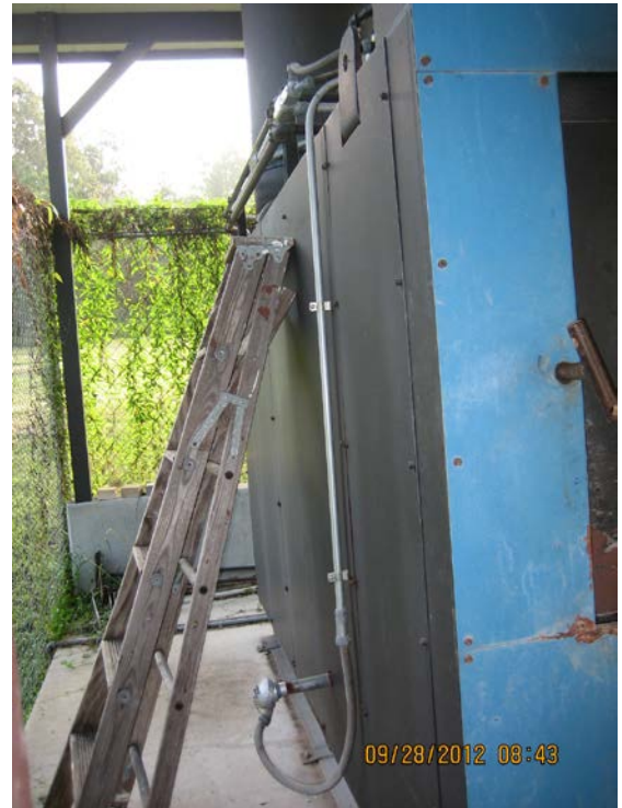
Photo ID No: IMG_436 – Primary Chamber thermocouple located on left side of cremation unit.
