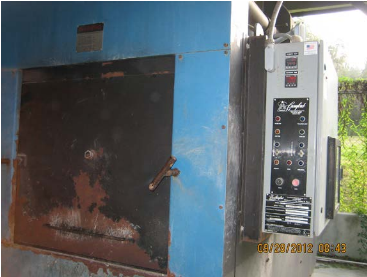
Photo ID No: IMG_435 - photo shows front view of cremation unit. The unit is a Crawford C700P cremation unit.
