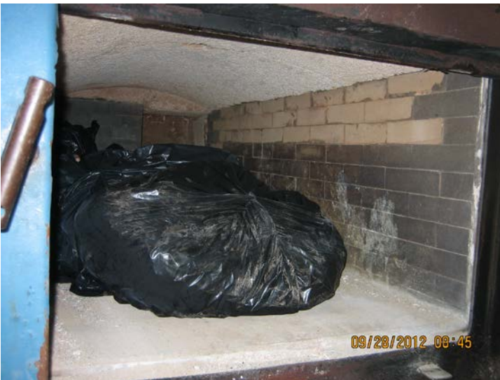
Photo ID No: IMG_439 – This facility does use bag containers during cremation. This photo was taken as the unit was being loaded for the Visible Emissions Testing.
