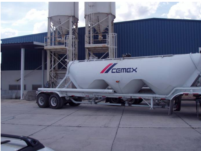
Photo ID No: 1050350_Photo_01_24_2012-16 Time: Approx 14:25 PM View of truck loading grey cement into South silo (EU005), camera facing approx. W. The white cement truck is behind the grey cement truck in the photograph.
