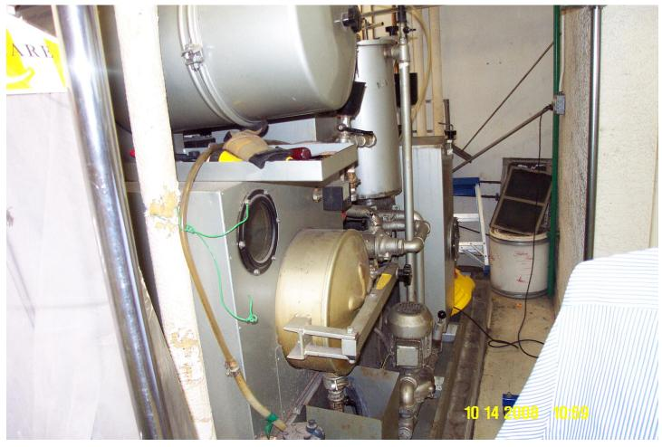
Project Id:66962Permit No: 1030424-004-AGArms Number: 0424Inspector:Shea JacksonInspection Date: 10/14/08Source (EU):New, Small Perchloroethylene Dry Cleaner: One Dry-to-dry machine (4/98-<br/>Aero Tech) with a refrigerated condenser, and 1 25 HP natural gas fired boiler.Description:-The rear area of machine clean no Perc odors detected containers in
