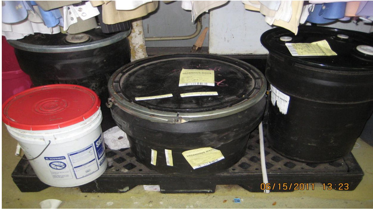
Photograph of Hazardous Waste drum Storage. Labels were properly displaying accumulation start Days and Drums were accessible.
