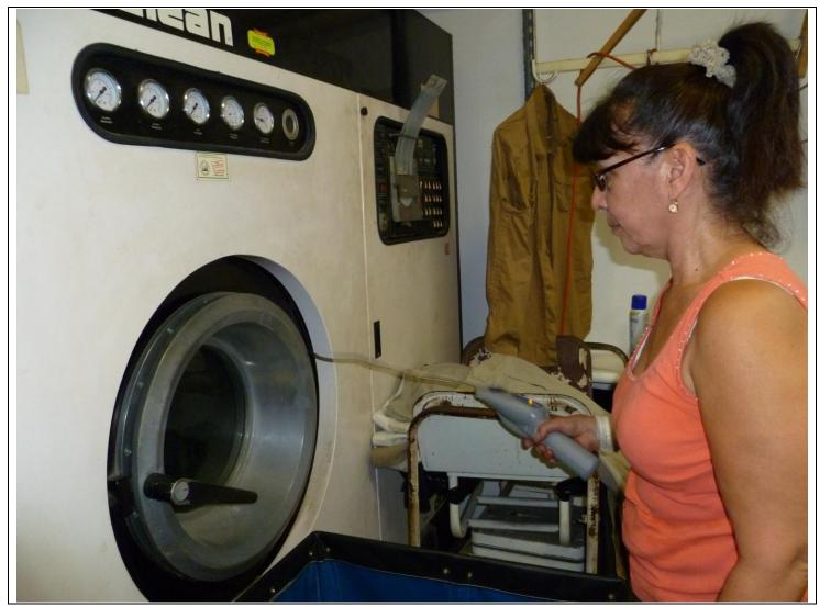
**Description:** [The responsible official demonstrated use of the halogen leak detector, going around the door, alarm detected a Perchloroethylene leak]
