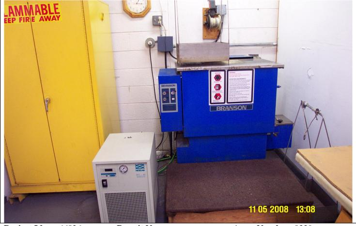
Project Id:66826Permit No: 1030329-003-AGArms Number: 0329Inspector:Shea JacksonInspection Date / Time: 11/5/08Source (EU):Existing, Halogenated Solvent Degreasing: Consists of onebatch vapor degreaser, purchased on 9/28/85, with a solvent-air interface area of <1.21 m2.</td>Facility uses 1,1,1-trichlorethane
