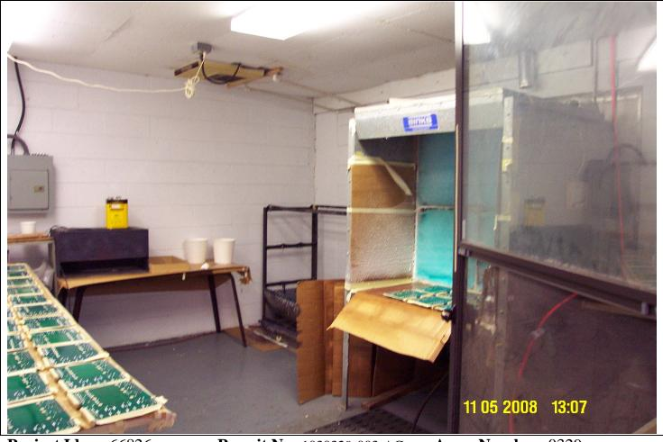
Project Id:66826Permit No: 1030329-003-AGArms Number: 0329Inspector:Shea JacksonInspection Date / Time: 11/5/08Source (EU):Existing, Halogenated Solvent Degreasing: Consists of onebatch vapor degreaser, purchased on 9/28/85, with a solvent-air interface area of <1.21 m2.</td>Facility uses 1,1,1-trichlorethane
