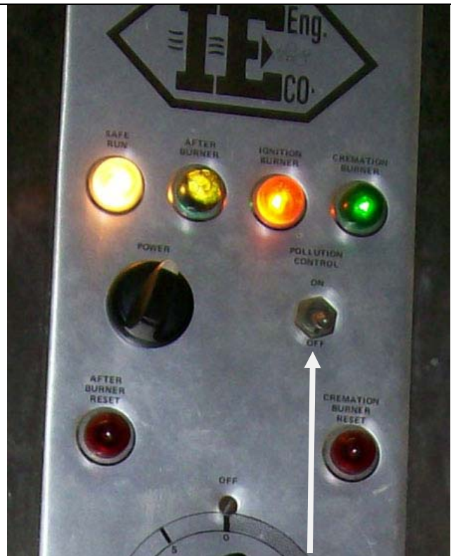
Note pollution control switch in off position
