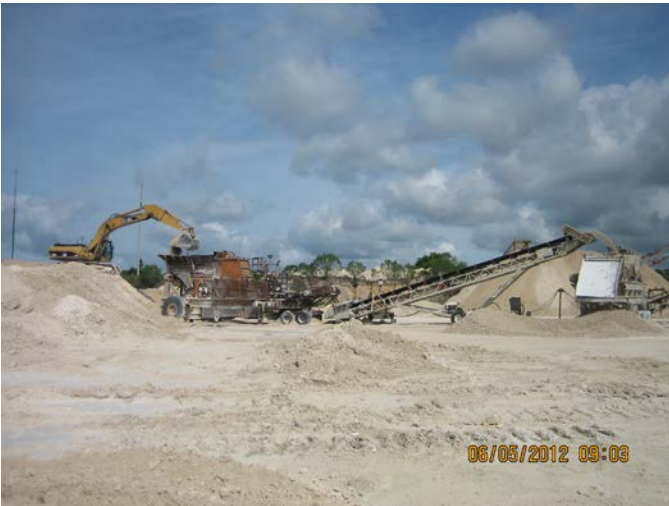
Photo ID No: IMG_426 – Facility ID No. 7774814: Hewitt Robbins Crusher (on left). Manufactured 1975. Power Screener Facility ID No. 7775703 on the far right.
