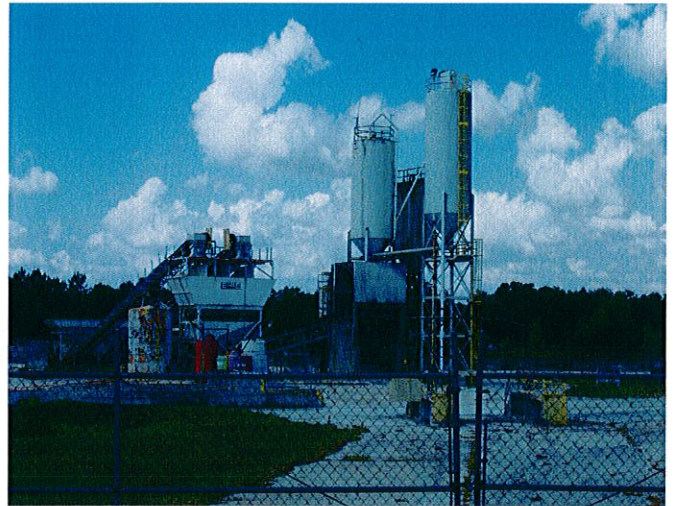
Photo ID No. / Date / Time: Picture 002 05-26-2011 11:15 Inactive silos and weigh hopper on facility grounds.
