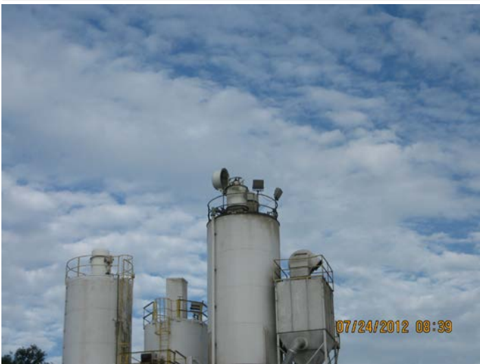
Photo ID No: IMG_449 – This photo is a close-up view of the Emission Unit No. 11 dust collector once release had stopped.
