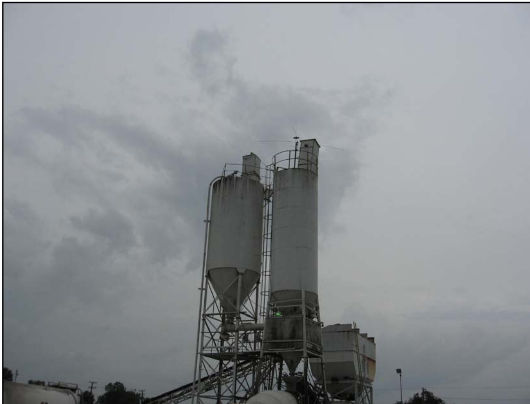
Photo ID No. / Date / Time: IMG_1439 / 06-06-12 / 0823 Slag silo (EU 002) on the left and cement silo (EU 001) on the right, during loading of the silos
