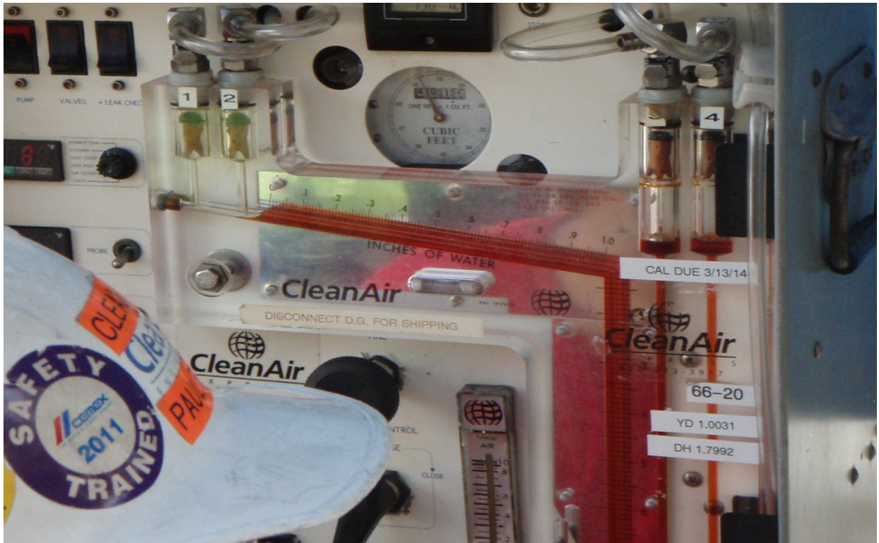
Stack Testing Equipment during Leak Check
