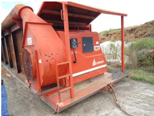
Back end of unit on skids showing diesel engine and heavy duty fan.
