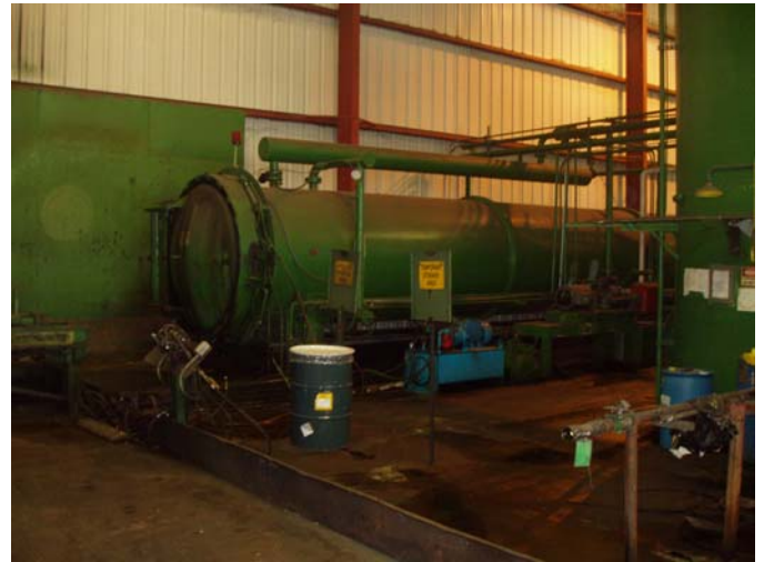
Photo ID No: 1190048_Photo_03_01_2012-002 Time: Approx. 10:00 AM Horizontal cylinder (cylinder 3) used for pressure treating wood products with CCA. The camera is facing approx. NW.
