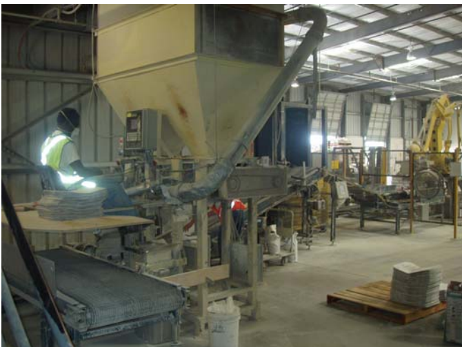
Photo ID No: 1050386_Photo_05_11_2012-004 Time: Approx. 10:45 AM Original packing machine (operating) and dust pickup line (diagonal gray pipe on side of machine). An operator can process two bags of finished material at a time by hand-feeding bags to machine. Camera is facing approx. NW.
