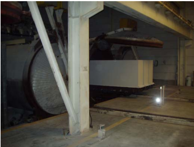
Photo ID No: 1050276_Photo_05_10_2012-011 Time: Approx. 11:15 AM Some of the autoclaves at the facility. The camera is facing approx. SW. The third autoclave (from East to West) is open with a load of concrete products sticking out. The fourth autoclave (from East to West) is barely visible in the photograph and is not connected and not operating.
