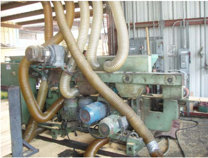
Photo ID No: 1050244_Photo_05_15_2012-008 Time: Approx. 12:00 PM Dust pickup points from sawing and moulding operations. The camera is facing approx. NE.
