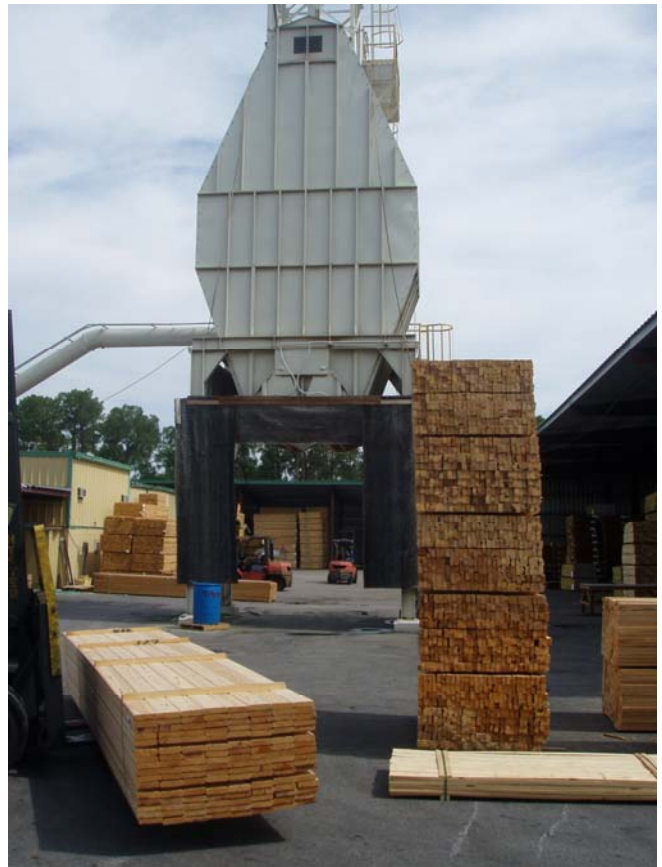
Photo ID No: 1050244_Photo_05_15_2012-002 Time: Approx. 10:45 AM Photograph of the sawdust storage silo. The camera is facing approx. N. Rubber curtains, to minimize fugitive dust emissions while loading sawdust into a truck, are on the South face of the truck loading area. The area appeared to be clean and well maintained.
