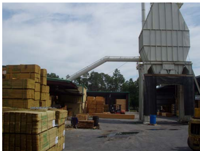
Photo ID No: 1050244_Photo_05_15_2012-004 Time: Approx. 10:45 AM Main sawdust pickup line from facility sawing operations to cyclone and sawdust storage bin. The camera is facing approx. N.
