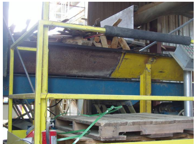
Photo ID No: 1050128_Photo_03_29_2012-006 Time: Approx. 12:15 PM Waste wood ready to be loaded onto the mechanical shaking pad that leads to the hammer hog; located inside hammer hog building. The camera is facing approx. SE.
