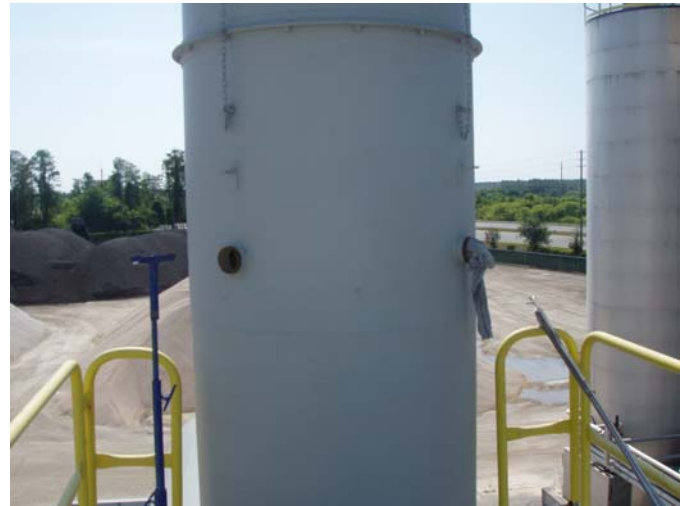
Photo ID No: 1010027_Photo_04_10_2012-011 Time: Approx. 11:00 AM View of the two stack port holes on the stack, where the probe is used to conduct the stack test. During testing, the port hole not used for each portion of the tests would be covered with a rag. The camera is facing approx. E.
