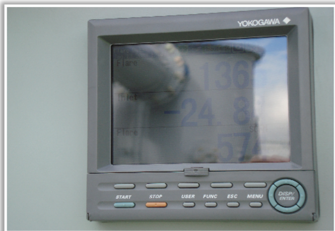
Photo 7: Display depicted in photo 5 showing -24.8 vacuum and 1365 degree F flare temperature
