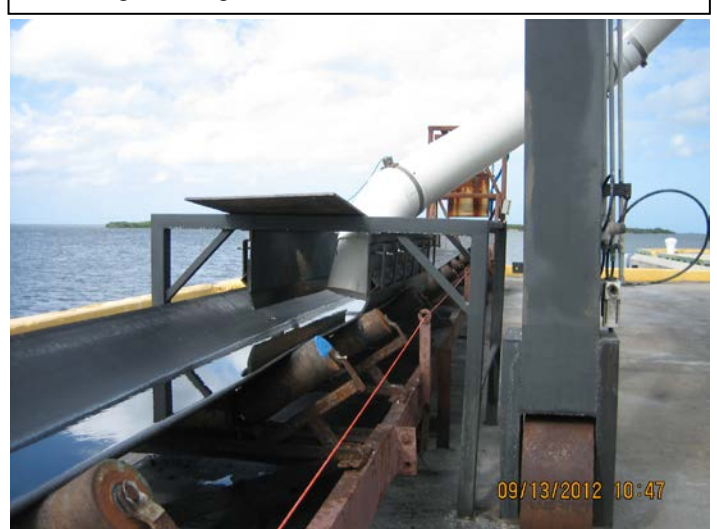
Photo ID No: IMG_432—Emission Unit No. 013 for Ship Unloading to Storage (New Hopper) drop point to conveyor.
