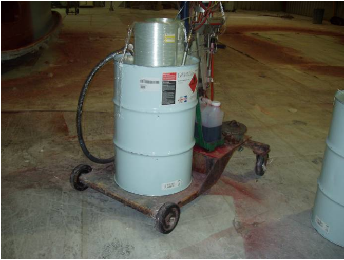
Photo ID No: Photo_0530363_02_23_2012-5 Time – Approx. 11:00 AM Cart carrying raw materials for chop gun, including resin, which is in the white barrel, fiberglass rolls, which are sitting on top of the resin, and catalyst, which is the red material inside the jug next to the resin. The camera is facing approx. N.
