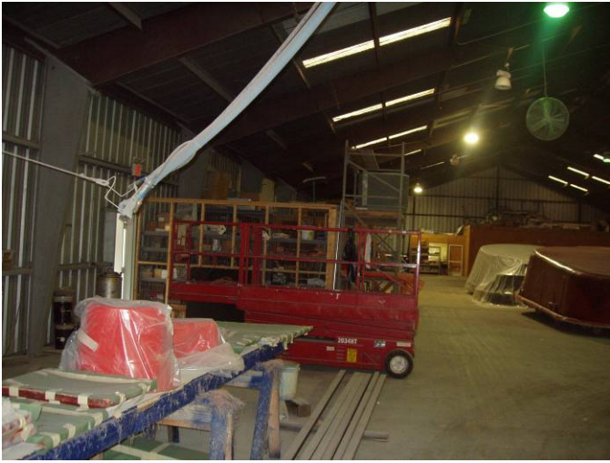
Photo ID No: Photo_0530363_02_23_2012-13 Time – Approx. 11:15 AM Pool mold repair and maintenance area. The grey cable hanging diagonally in the foreground of the photograph is a vacuum connection for the Eurovac III system. The camera is facing approx. S.
