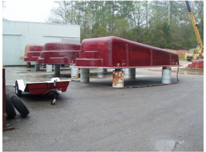
Photo ID No: Photo_0530363_02_23_2012-7 Time – Approx. 11:00 AM Location at the facility where the perimeter of each pool is trimmed using hand tools equipped with vacuum devices to capture dust. A crane visible in the background of the photo is used to lift each finished pool out of its mold. The camera is facing approx. NW.
