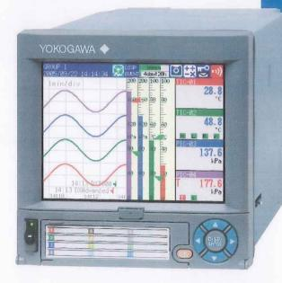
The new DXAdvanced DX1000N features an inner chassis that can be removed from the case via the front panel of the instrument. This provides access to all of the internal components of the **DX1000N** from the control panel without having to access the rear of the unit or disturb any of the field and power supply wiring. Functionality, appearance, and panel cutout dimensions are the same as those of the standard DX1000.
